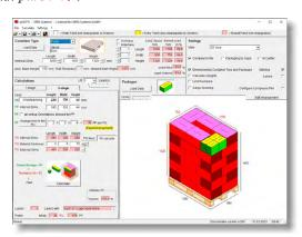
Individually Adaptable, Exact Analysis in 2D and 3D Import, edit and save container types, package data, outer packages and other preferences imported from any data file, e.g. server file Consideration of base height and wall thickness, allocation of substructure or overhang of the container type
